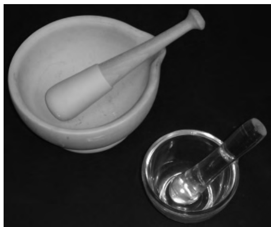
Figure 2.1 A porcelain mortar and pestle and a smaller glass mortar and pestle.
