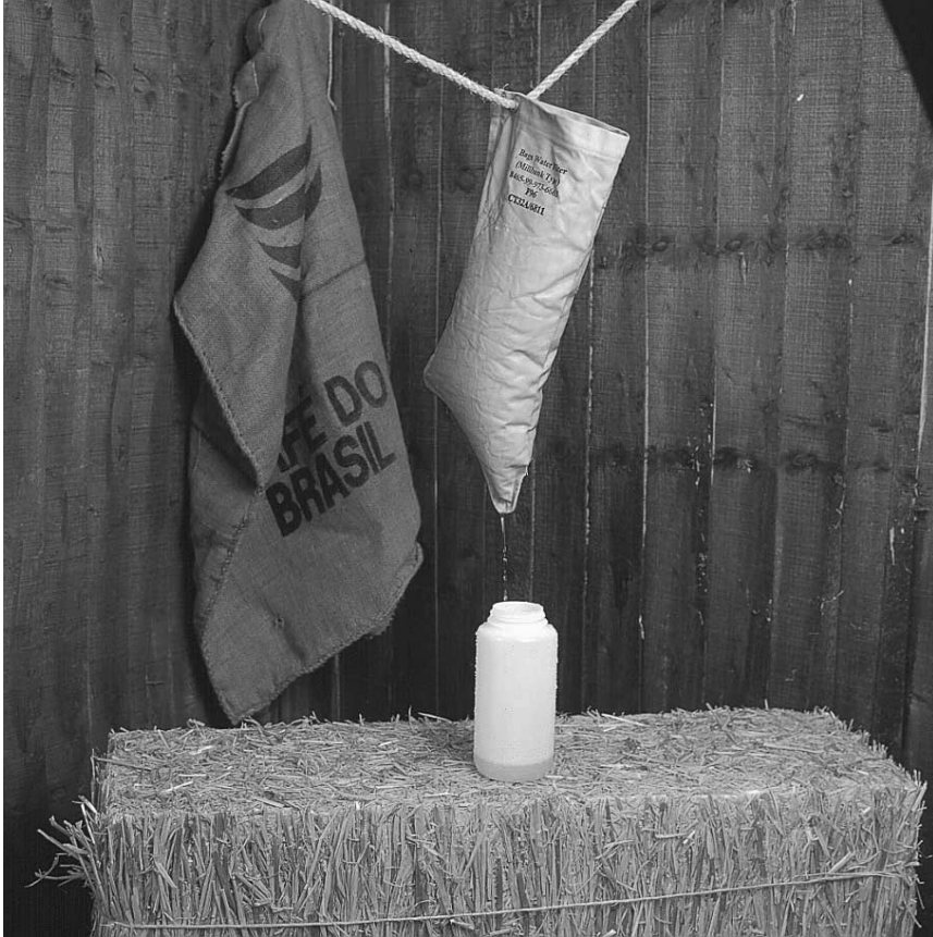
Figure 3.1 Millbank bag for filtering water prior to chemical disinfection. Courtesy of Nomad.
